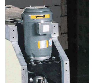
Hydraulic motor pump assembly mounted in left hand rear press bed leg.
