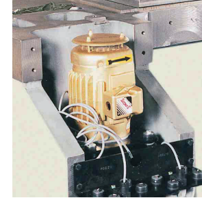
Lube motor pump assembly mounted in right hand rear press bed leg.
